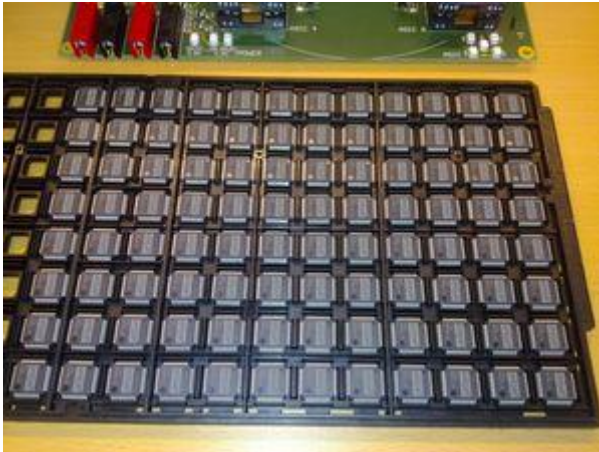
Title: UNIQUE ASICs Caption: 96 UNIQUE ASICs. Each chip includes 6 different PUF types. Copyright: UNIQUE Consortium
